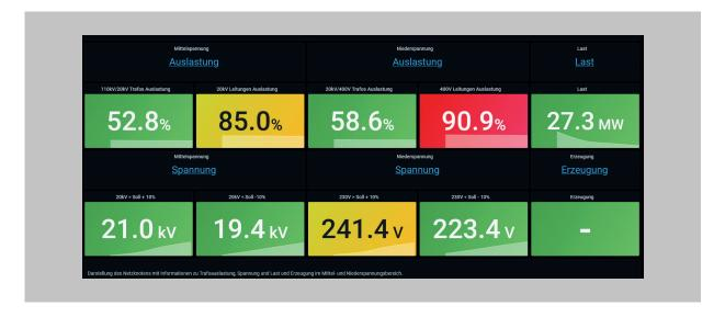
The ever-increasing share of volatile energy causes high loads on transformers in local area substations at peak times. These loads can be detected by monitoring the temperature of components installed. The installation of IoT-capable temperature sensors in stations concerned may indicate bottlenecks in good time and thus enable grid control systems to impose countermeasures that prevent sudden breakdowns.
